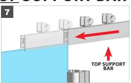
**SLIDE "TOP SUPPORT BAR" ALONG THE FABRIC TUBE**
