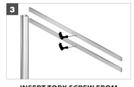
INSERT TORX SCREW FROM STEP1 AND TIGHTEN
