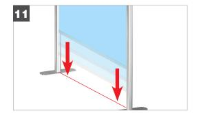
**KEEP WORKING SUPPORT BARS** AND FABRIC TILL BARS REACH TOP **AND BOTTOM EVENLY** WITH SUPPORT POSTS
