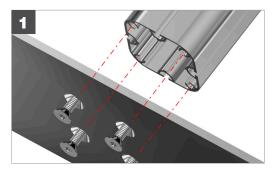
INSERT SCREWS INTO BOTTOM POST
