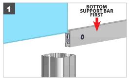
**SLIDE FABRIC TUBE INTO BOTTOM SUPPORT BAR CHANNEL FIRST**
