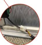
**3).** Lay out the wire harness across the bottom of the frame and plug it into the controller.
