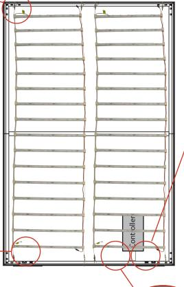
**2).** Install the controller on the backside of the frame. Plug the barrel connector from the controller and all the light curtains into the into the corresponding power supply.
