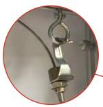
1.) Adjust top hooks so they are 3" from the top of the board. Hang the lights in front of the support bars with the open side of the hook and the LEDS are facing out. Next hook the bottom of the light through the eyelet and pull cable to tighten the lights.
