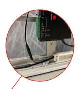
**2).** Install the controller on the backside of the frame. Plug the barrel connector from the controller and all the light curtains into the into the corresponding power supply.
