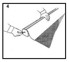
Grip the image and display with your left hand. Remove the locking pin with your right hand. **THE SPRING IS NOW ACTIVATED!**
