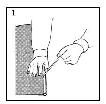
Always make sure the surface is clean. Place the image (picture side up) to the top profile. Remove the protective strip and then press firmly!
